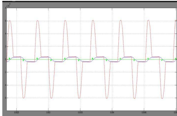
Fig.14. simulation waveform of resonant inductor current i_{Lr} , capacitor voltage and capacitor Current for 1MW
